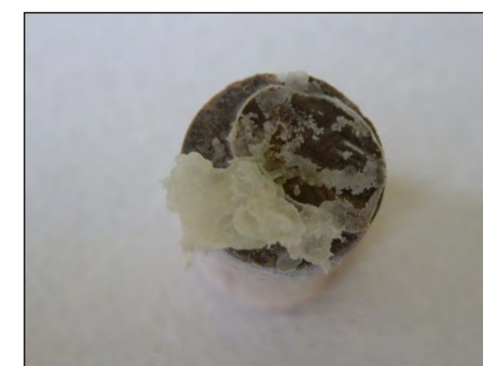
Fig. 3: Photos of archive Portland cement paste (old borehole filling) before and after spCO 2 exposure.
