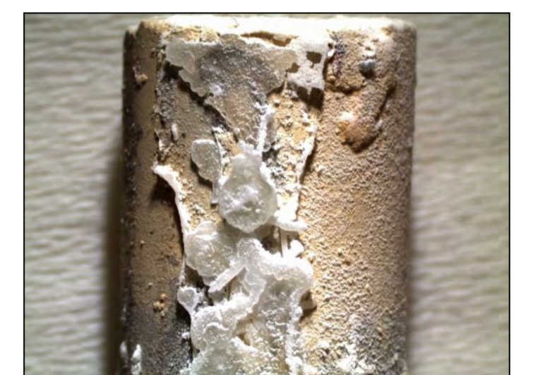
Fig. 4: Photos of mixed cement paste CEM II. (recent borehole filling) before and after spCO 2 exposure.
