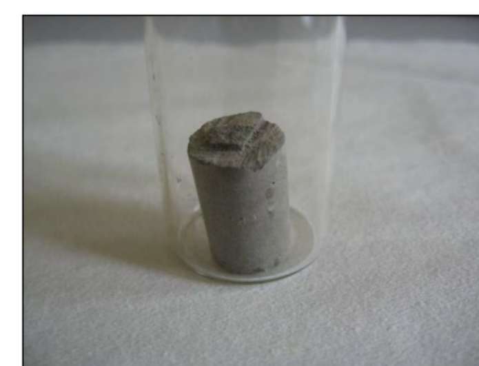
Fig. 3: Photos of archive Portland cement paste (old borehole filling) before and after spCO 2 exposure.
