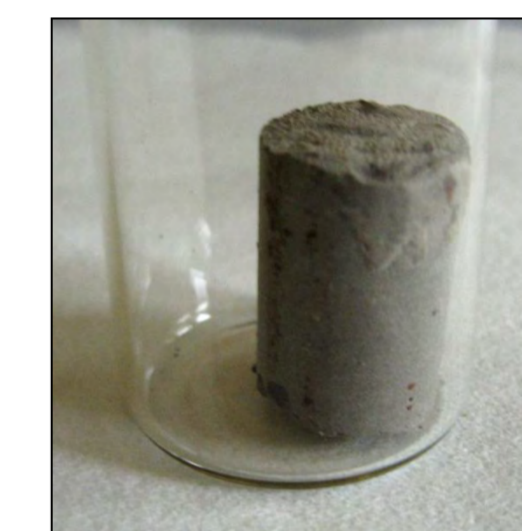
Fig. 4: Photos of mixed cement paste CEM II. (recent borehole filling) before and after spCO 2 exposure.
