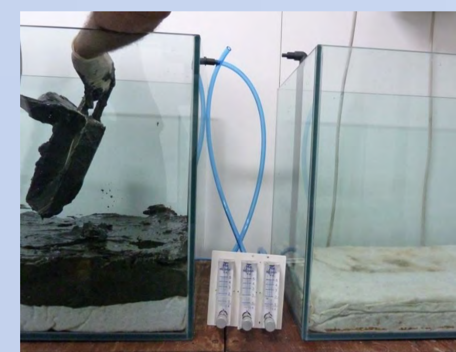
Disposal of contaminated sediments into the containers.
