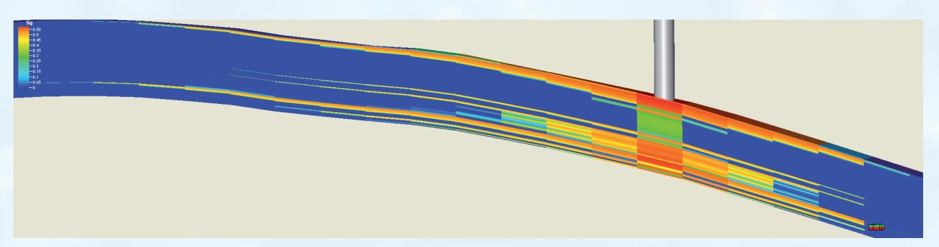
Vertical section through injection well. CO<sub>2</sub> gas phase saturation after 10 years injection. Section 4 km long, 300 m height.
