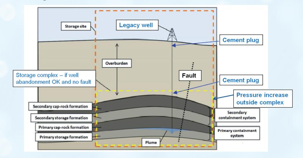
The figure shows a principal sketch for the Vedsted site defining the storage complex and the different site specific conditions that were considered. There seems to exist some confusion in the definition of storage site and storage complex; in the definition of the storage site the surface facilities are included, but the complex may be defined without including the surface if wells penetrating through the overburden are properly sealed off.
