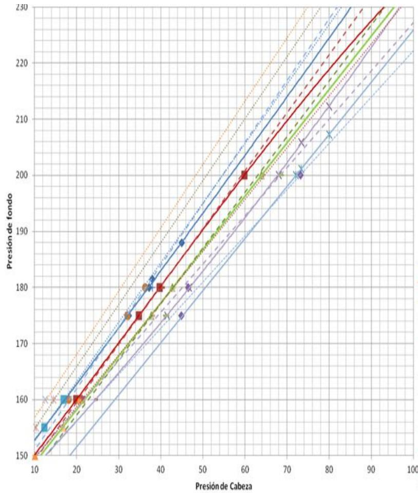
The injectivity abacus correlates the WHP with the WBP and the injection flow per each reservoir operational stage, this means the correlated parameters could change during the different phases of the project.
