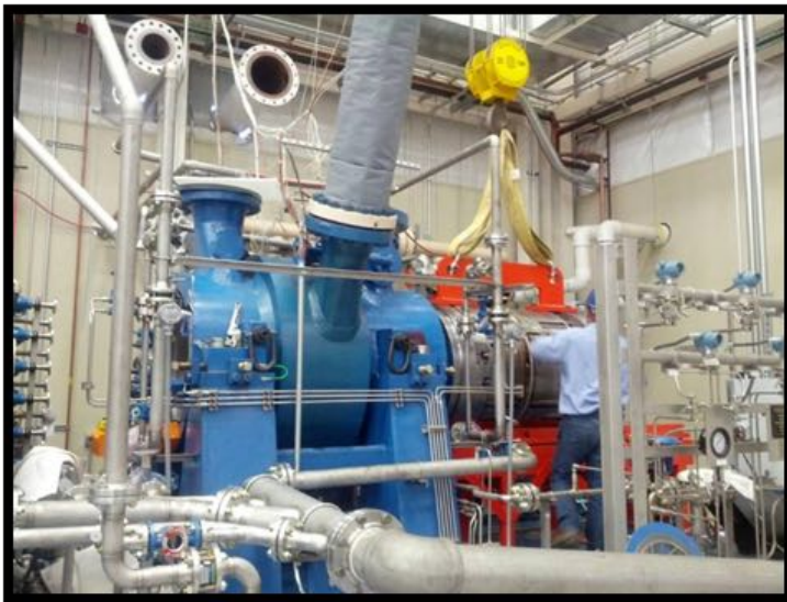
Dresser-Rand 6-stage CO 2 Compressor with Generation-2 Cooled Diaphragms
