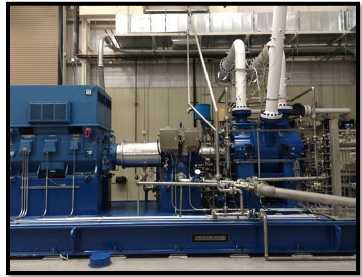
Dresser-Rand 6-stage CO 2 Compressor with Generation-2 Cooled Diaphragms
