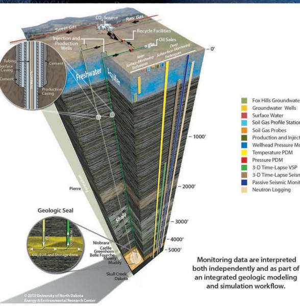
Fox Hills Groundwater Wells Groundwater Wells Surface Water Soil Gas Profile Stations Soil Gas Probes Production and Injection Rates Wellhead Pressure Monitoring **Temperature PDM** Pressure PDM 3-D Time-Lapse VSP 3-D Time-Lapse Seismic Passive Seismic Monitoring Neutron Logging
