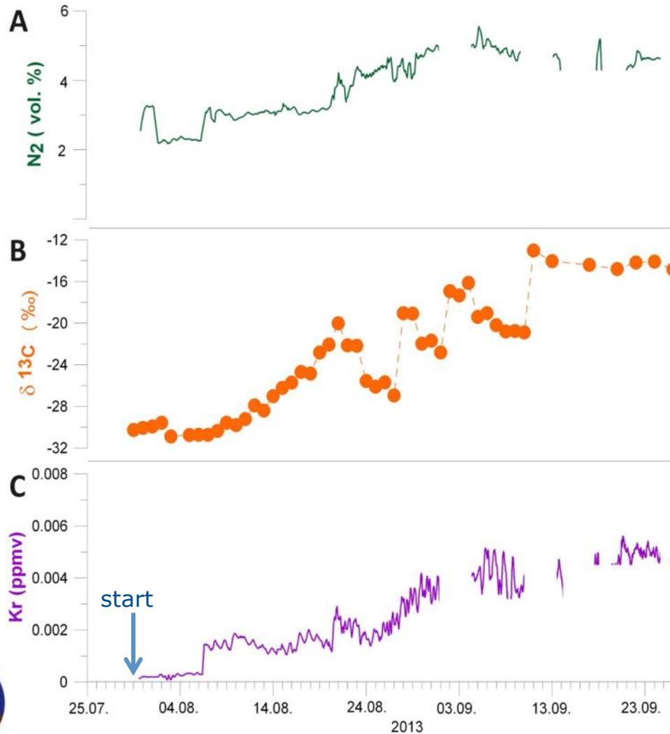
→ gas mixture arrived after about 4 days at Ktzi 203 ~20 m from injection well Ktzi 201
